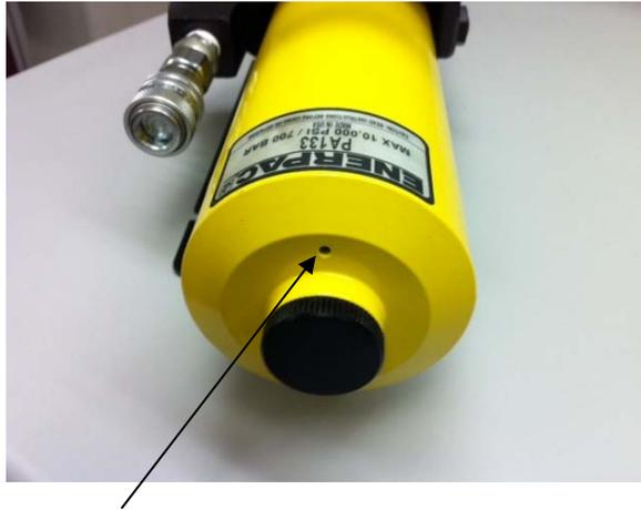
Note the small vent hole on the end of the pump. If you verified the nuts on the pump rocker switch are tight (step 7), and the pump is still not building pressure, try the following:
